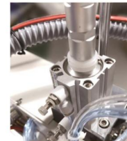
上柱行程可调 Easy adjust Upper column route
